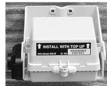
Close up view of one of YCUA's new Meter Transceiver Units (MXUs).
