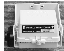
Close up view of one of YCUA's new Meter Transceiver Units (MXUs).
